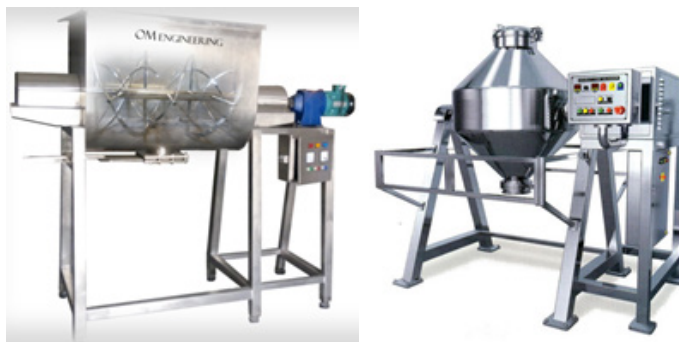
Fig. 3.26 Mixers (a) ribbon blender(b) double-cone mixer
