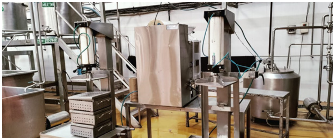
Fig. 3.31 Vacuum Sealing Machine for Sweets
