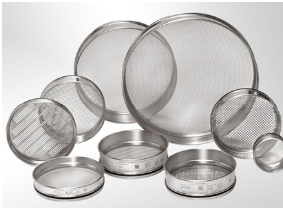
Fig. 3.1 Screening of dry materials
