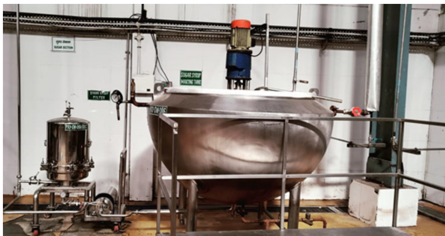
Fig. 3.45 Steam Kettle used in Sweet Industry
