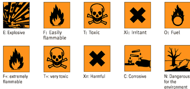
Fig. 5.17: Chemical hazard safety signs
